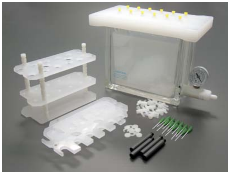
12-position Vacuum SPE manifold (p/n SPE-5869-000A)
