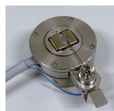
Heating holder * Sample size 10 \times 15 \times 3mm * Temperature range R.T \sim 250 ^{\circ}\text{C} (High load) R.T \sim 180 ^{\circ}\text{C} (Low load)
