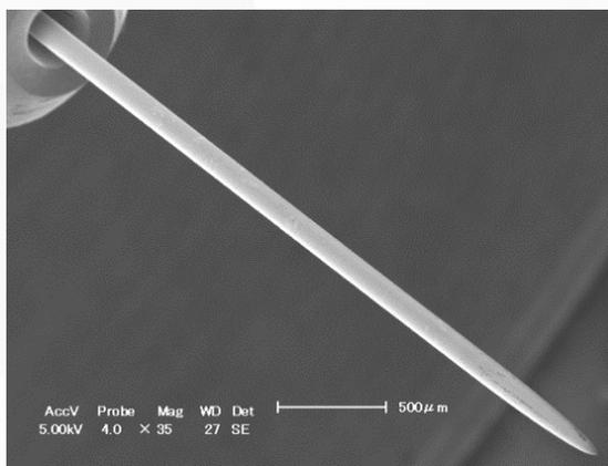
Fig.1 Scanning Electron Microscopy image of a PESI probe used in DPiMS.
