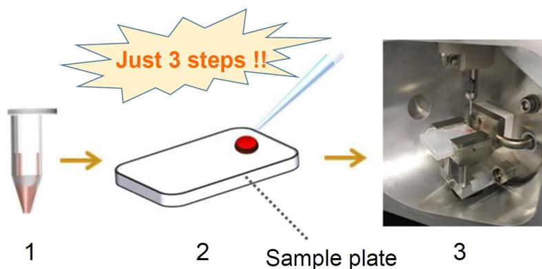
1. Whole blood (10  $\mu$ l) is diluted 10-fold with an IS\* (50 ng/ml) aq. Then the diluted solution is further diluted 2-fold with ethanol.
