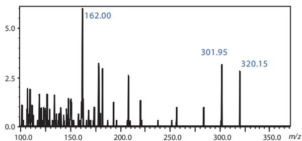
Fig. 3 Product Ion Scan of TTX Standard Sample
