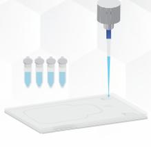
Liquid samples can be crude but ionization occurs more efficiently after appropriate dilution. Spot samples directly into a disposable liquid sample plate.
