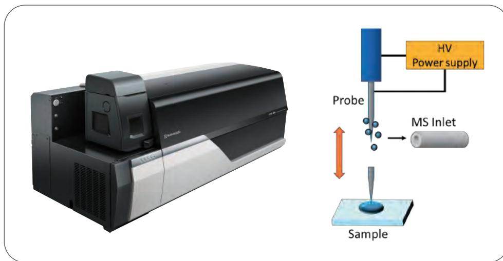
Figure 1 DPiMS-8060 and LCMS-8060 triple quadrupole mass spectrometer
