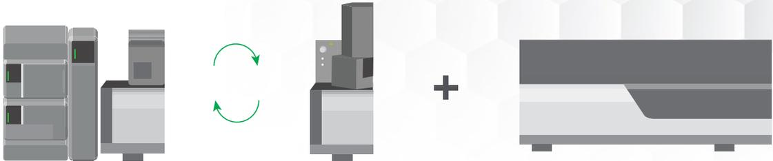
The ionization unit of DPIIMS can be detached and replaced with the heated ESI unit to enable LC/MS analysis using the same MS hardware and operating software. Switching takes only a few minutes without the need for special tools or service engineers.
