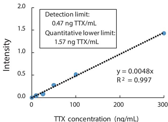
Fig. 4 Calibration Curve of TTX Standard Sample
