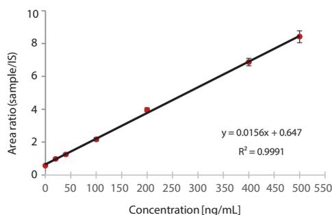
Fig. 4 MT-45 Calibration Curve by Standard Addition
