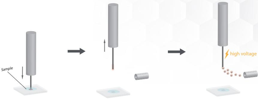
i) The probe is first lowered into the sample.
