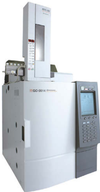
Shimadzu GC-2014 for measurement of alcohol content
