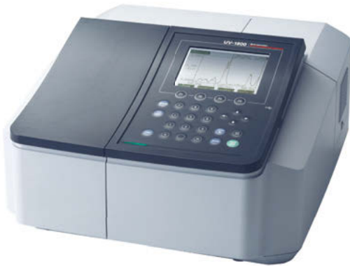
Shimadzu UV-1800 for measurement of beer IBU and color
