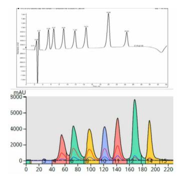
**Figure 1.** A method developed on an HPLC using a C18 scaling column (top) and the flash chromatography results using the same method on a 12-gram Sfär C18 column (bottom). The separations are nearly identical.
