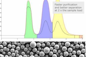
Irregular silica 50 µm, 25 g column, 25 mL/min, sample loading 2% wt/silica.
