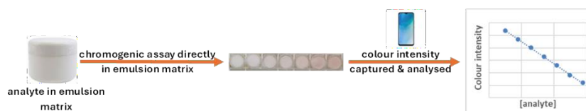
Fig. 1. Setup for the proposed extraction-free quantification methodology
