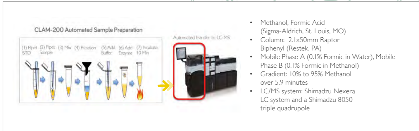
Figure 1. Sample preparation and analysis on CLAM-2000 and LCMS 8050
