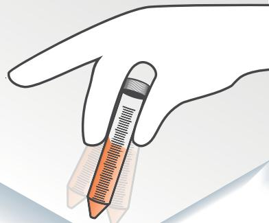
10. Centrifuge for 5 min at 3000 rpm
