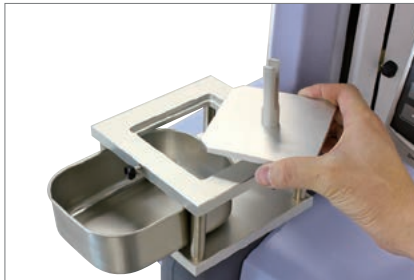
① Jig platform
