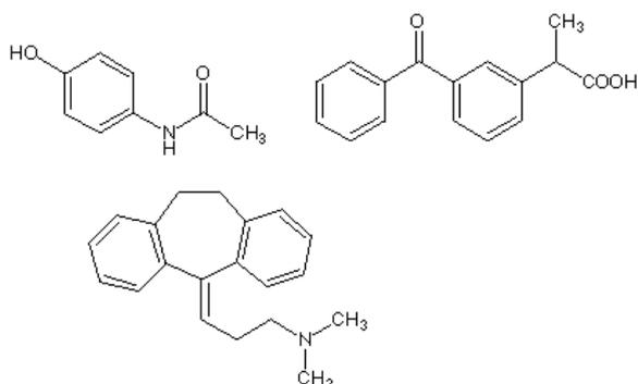
Structures of acetaminophen (neutral), ketoprofen (acidic) and amitriptyline (basic): examples of the broad range of analytes extracted in this application.
