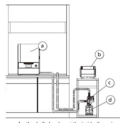
Please prepare for the draft chamber at the inside dimension of more than D650  $\times$  W1000  $\times$  H60 (mm). Sirrocco fan: CES-V
