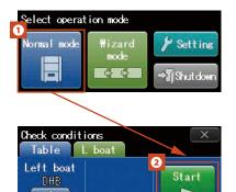
After system startup, press (1) and then (2) to start deposition.
