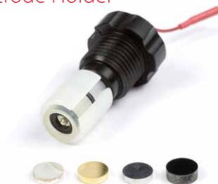
Working electrode holder (assembly) with supplied electrodes: Pt, Au, GC and MD (left to right).
