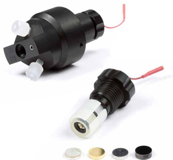
(MD), which can be quickly and easily exchanged. Magic Diamond (MD) also known as Boron Doped Diamond (BDD) is the workhorse and electrode of choice for oxidation reactions up to a maximum applicable voltage of 4.0 V. Pt and Au are typically employed for specific reactions such as hydroxylation or N-oxidation.
