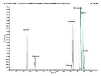
Extracted ion chromatogram of antiepileptic drugs.
