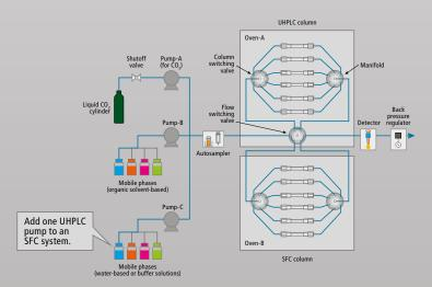
SFC and UHPLC involve significantly different mobile phase and separation characteristics, but stable analysis can be performed in either mode, by purging the flow lines with the respective eluent used. This washing and equilibration step is accomplished by executing a pre-defined batch table generated automatically by the dedicated software. The streamlined process is easy-to-use, even for non-experts, for smooth switching between SFC and UHPLC analyses.
