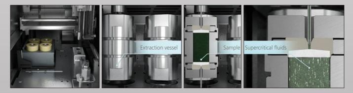
The Nexera UC online SFE-SFC approach eliminates the need for tedious, manual sample pretreatment. Combined with MS, it offers quick and easy on-line sample extraction with state-of-the-art chromato-graphic separation and high sensitivity detection.
