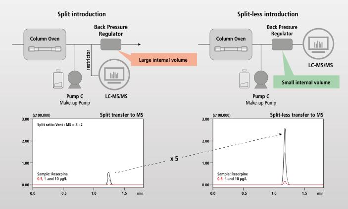
The simple, elegant design allows for easy maintenance. With a dispersion volume of less than 1  $\mu$ L and integrated temperature control, the SFC system can be connected directly to a mass spectrometer without the need for a special interface or flow splitter. The introduction of the entire amount of eluent has the potential to significantly increase MS sensitivity.
