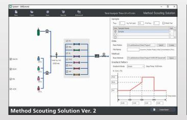
With the dedicated "Method Scouting Solution" software, various analytical conditions can be applied simply by selecting them from the graphical user interface (GUI). It supports an automated workflow by calculating analysis run time, modifier and sample amount required, automated method and batch creation as well as prevention of degradation through column rinsing.
