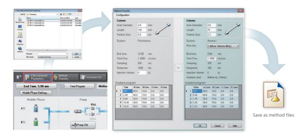
The Nexera-i MT has two flow lines matched to the UHPLC and HPLC delay volumes. In addition to simplifying method transfer for customers using HPLC, this single integrated system also streamlines reviewing procedures for increasing the speed of customers' methods using UHPLC.
