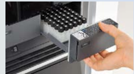
Rack can be pulled out even when needle is active
