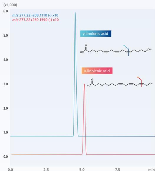
$\alpha$ -linolenic acid and  $\gamma$ -linolenic acid with different double bond positions were analyzed using Nexera UC and the OAD-TOF system. Isomers with similar structures were completely separated by SFC and detected with specific fragment ions derived from OAD, enabling highly accurate analysis. OAD can also be adapted to monovalent negative ions such as fatty acids.
