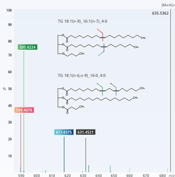
Lipids in butter were analyzed using DPiMS in combination with the OAD-TOF system. Specific fragment ions derived from OAD were observed with only a simple pretreatment, which is a feature of DPiMS, and the double bond position of triacylglycerol was quickly estimated.
