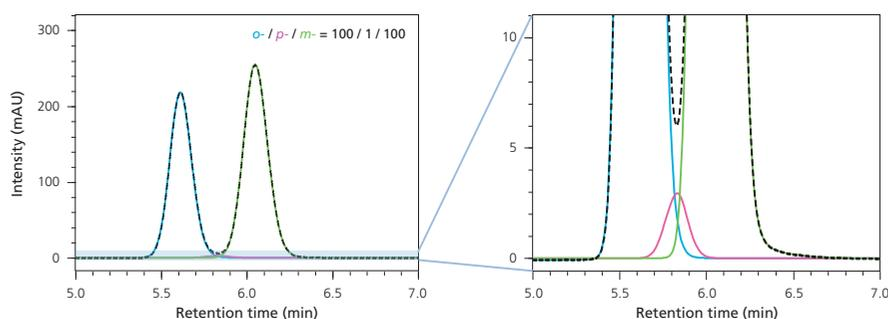
Fig. 4 Separation Results for Mixture Sample of *o*-MAP, *m*-MAP, and *p*-MAP
