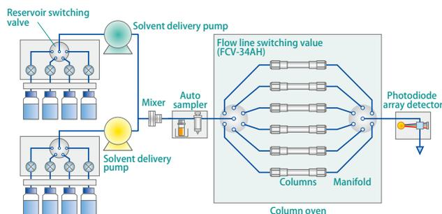
Fig. 2 Nexera Method Scouting System Flow Line Diagram
