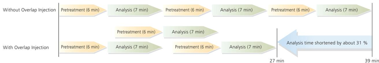
Fig. 11 Shortened Analysis Time Using Overlap Injection
