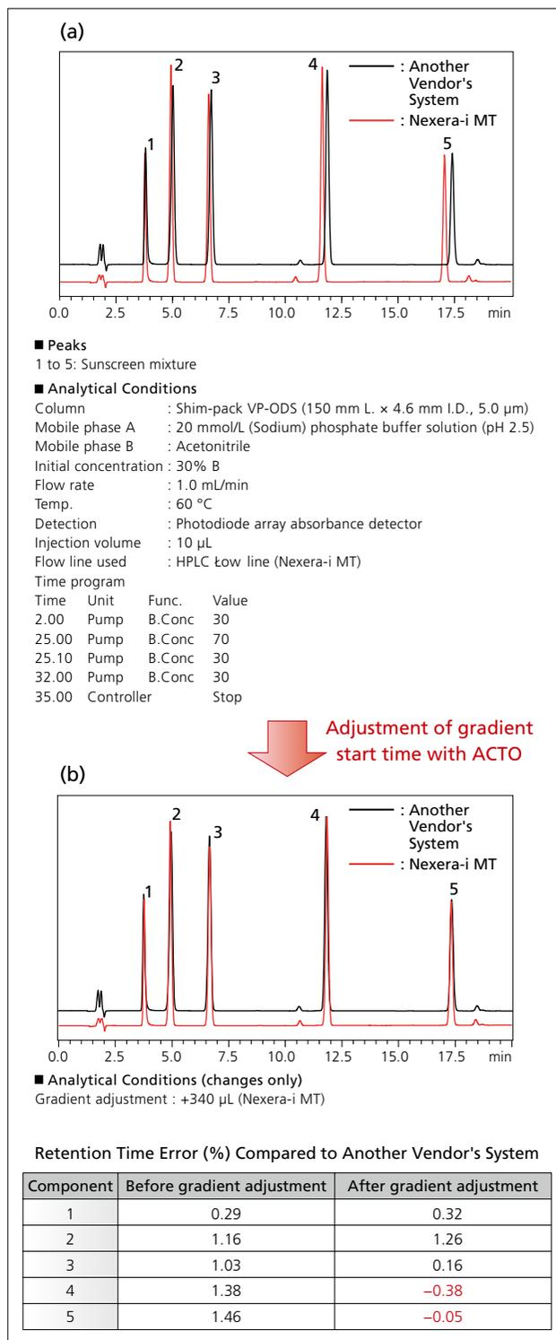
Fig. 5 Example Method Transfer with Gradient Adjustment (Sunscreen mixture)
