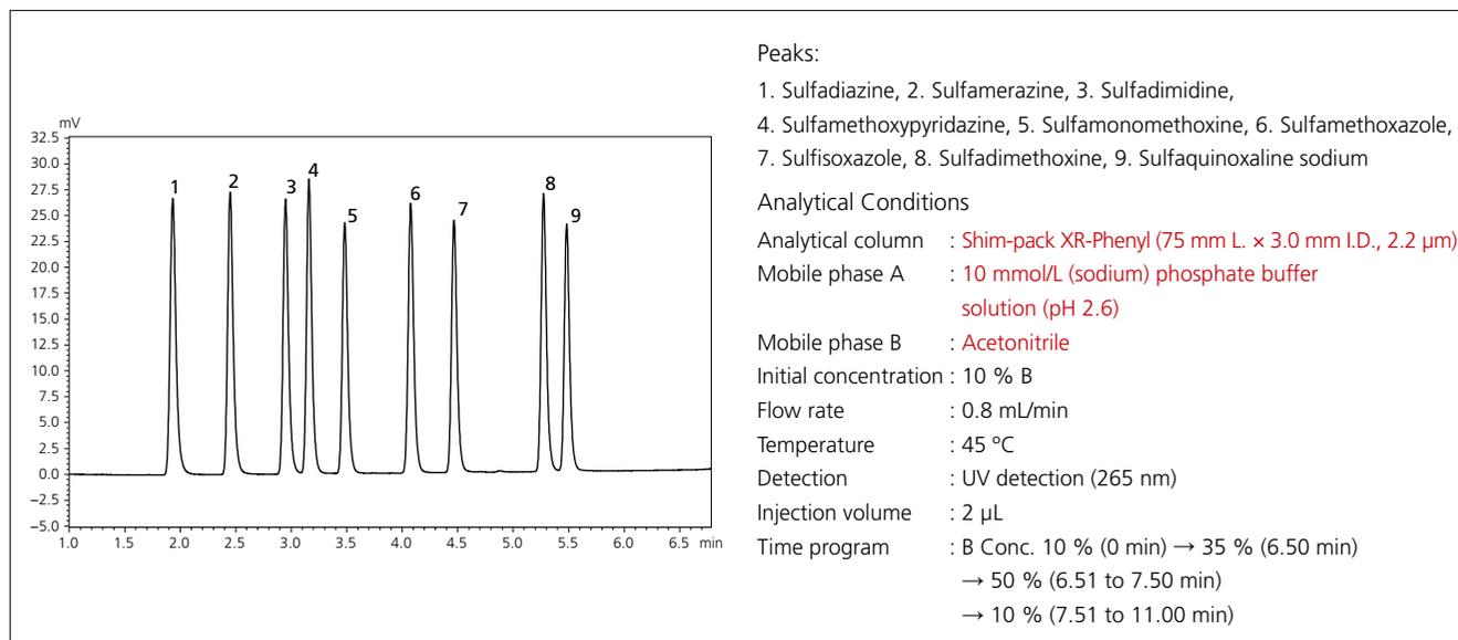
Fig. 12 Optimal Combination of Column and Mobile Phases for Simultaneous Analysis of Sulfa Drugs Determined by Method Scouting and Corresponding Chromatogram
