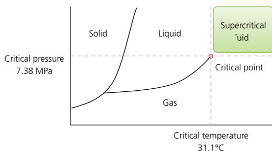
Fig. 1 Phase Diagram for Carbon Dioxide
