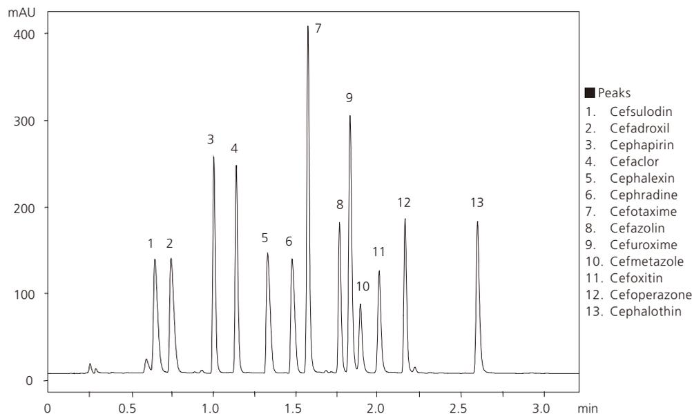
Fig. 12 Simultaneous Analysis of 13 Cephem Antibiotic Substances
