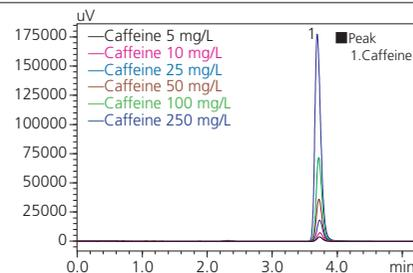
Fig. 4 Overlaid Chromatograms of Standard Solutions (5–250  $\mu$ g/L)
