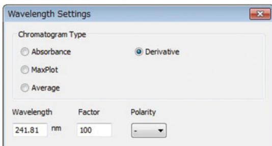
The derivative spectrum chromatogram has positive value when the slope of the spectrum is up and negative value when the slope of the spectrum is down. Peak direction in the derivative spectrum chromatogram can be adjusted by setting the polarity, and peak size can be adjusted by setting the factor.
