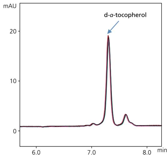
Results for SFE extraction liquid analyses of Vitamin E. The automated consecutive pretreatment of solid sample by the Nexera UC SFE pretreatment system showed both high repeatability and high recovery.
