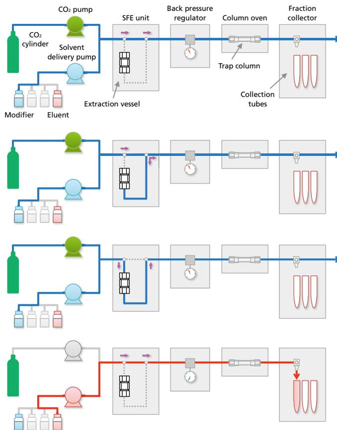
Fig. 4 Material Flow and Principle of Operation
