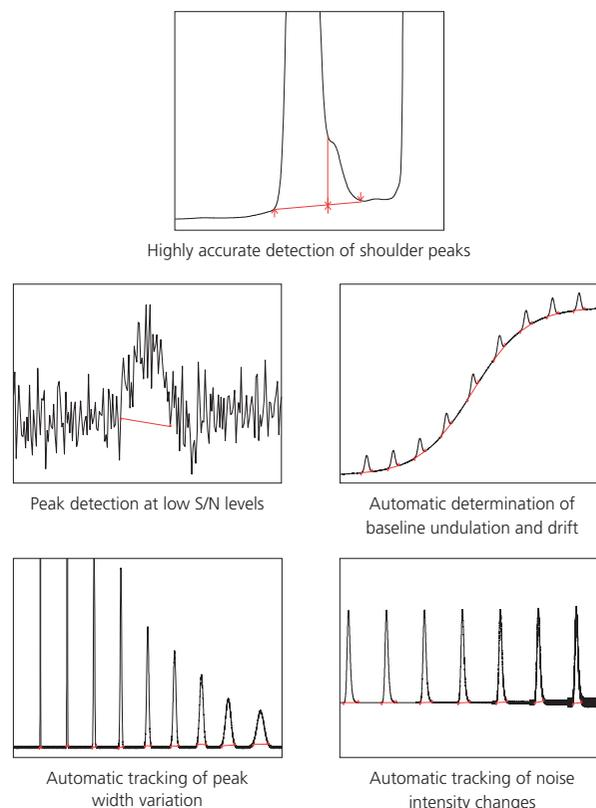
Fig. 1 i-PeakFinder's Completely Automated Integration Function
