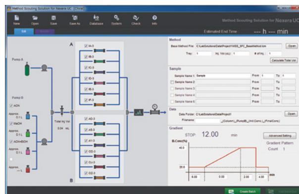
Fig. 11 Configuration Window of Method Scouting Solution Software
