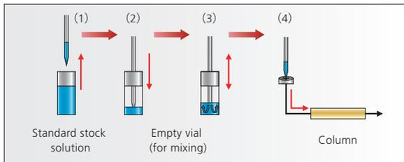
Fig. 2 Standard Solution Injection Operation Procedure
