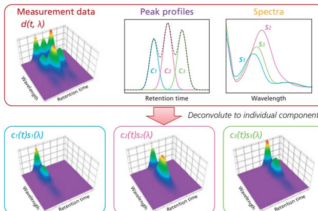
Fig. 1 Measurement Data from Three-Component Mixture Sample
