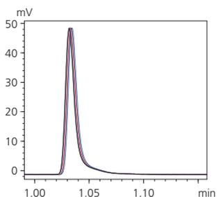
Fig. 5 Chromatogram with Peak Tailing (N=5)
