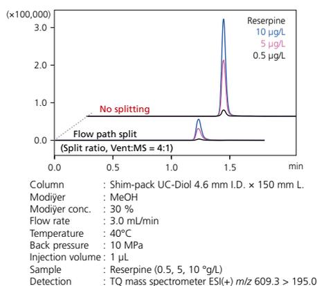
Fig. 8 Sensitivity With and Without Flow Path Splitting
