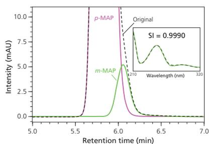
Fig. 5 Impurity Contained in *p*-MAP Standard Sample
