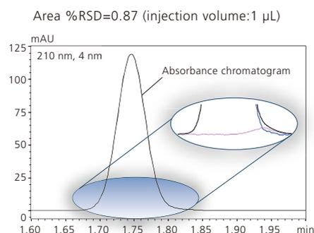
Fig. 6 Absorbance chromatogram of the mixed sample (DFBP/VP=100/1)
