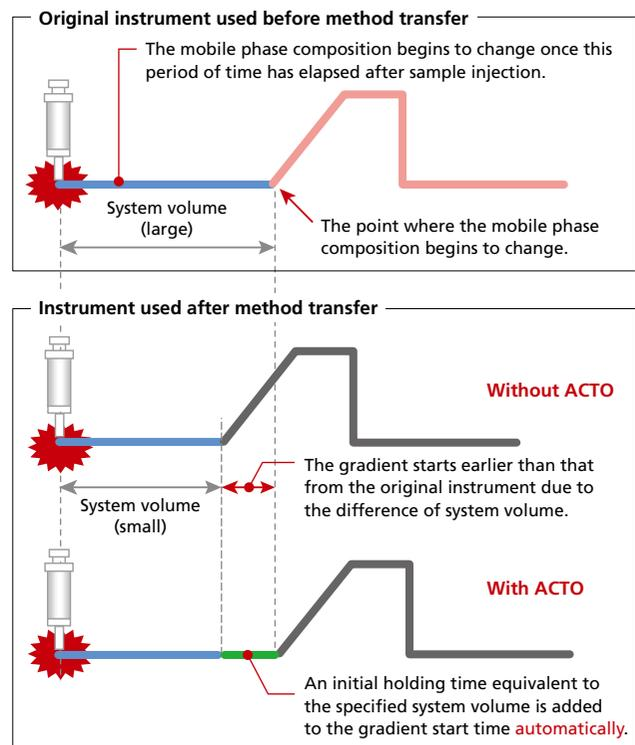
Fig. 7 Adjusting the Gradient Start Time
