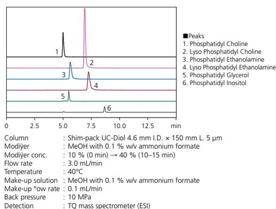
Fig. 9 Phospholipid Analysis
